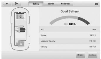
Figure 7-7 Sample Battery Test Results Screen
