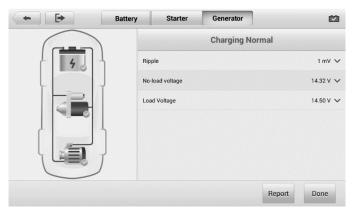
Figure 7-10 Sample Generator Test Results Screen Table 7-6 Generator Test Results
