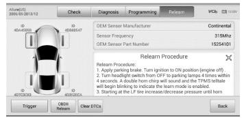
Figure 6-24 Sample Stationary Relearn Screen 1
