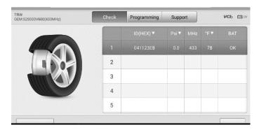
Figure 6-33 Sample Check Screen via OEM Part No.
